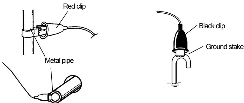
Note: Clean off if the connected part is rusted or painted to ensure a good electrical connection.
