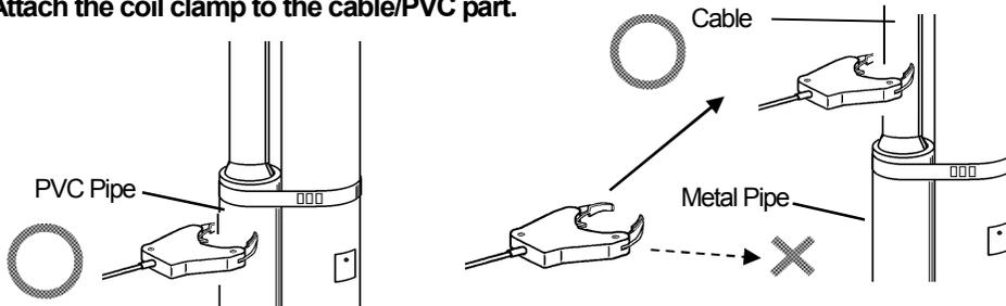
**Note :Use the Receiver more than 5 m/16 ft away from the coil clamp
