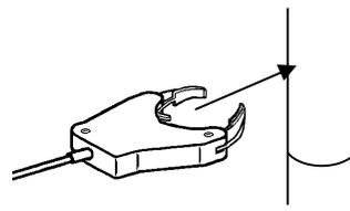
\*The jaws do not have to be closed around the cable.
