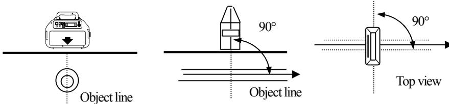
\*Location near the area of a manhole, place the Transmitter on the side of the manhole you wish to locate.
