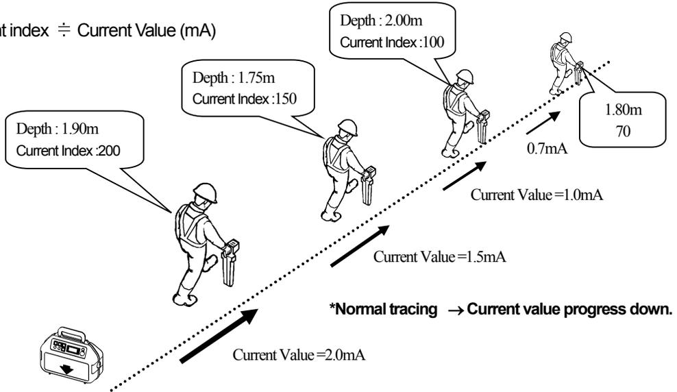
\*The Current gradually reduces as the distance from the Transmitter increases.
